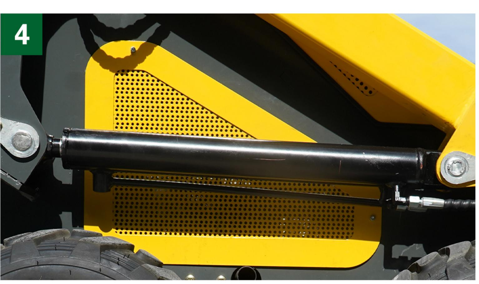
The inversion of the cylinder can effectively protect the cylinder rod from damage and prolong the service life of the cylinder.
