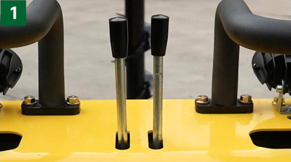
The auxiliary device operating lever has a self-locking function, which is more convenient to operate and saves time and effort.
