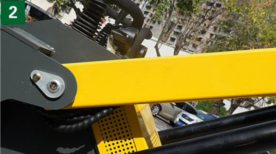
The oil pipe adopts a built-in pipe arrangement, which can effectively protect the oil pipe, reduce wear and tear and prolong the service life of the oil pipe.
