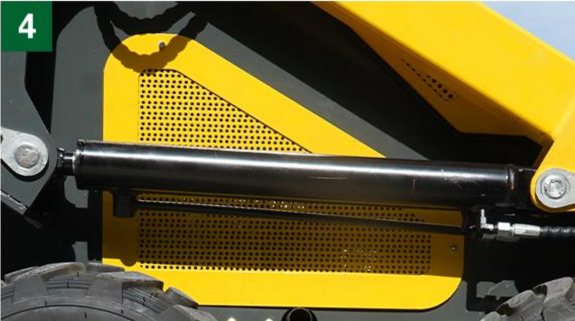
The inversion of the cylinder can effectively protect the cylinder rod from damage and prolong the service life of the cylinder.
