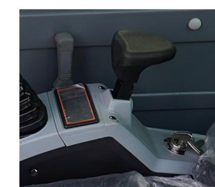
Bulldozer blade and starter key
