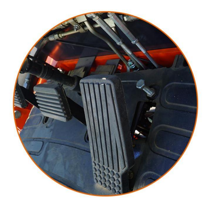
Suspended (type) pedals are used to provide extra foot space, which significantly reduces
