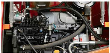
The large-opening hood can be opened upward  $90^{\circ}$ , providing a large space for maintenance; the air filter and fuel filter are centrally arranged.
