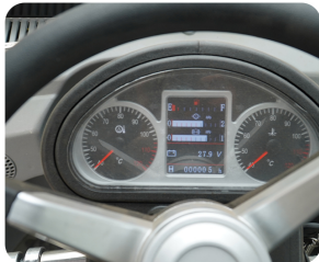
The instrument panel is simple and clear, making it easier to observe the machine status and drive experience.
