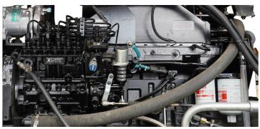
The large-opening hood can be opened upward  $90^{\circ}$ , providing a large space for maintenance; the air filter and fuel filter are centrally arranged.
